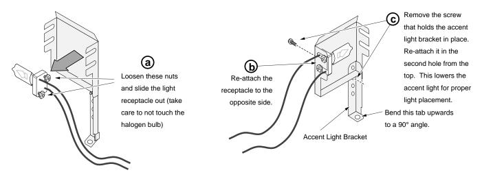
2 Remove the burner from the stove (see owner's manual for details). Install the accent light assembly as shown in the illustration below.
