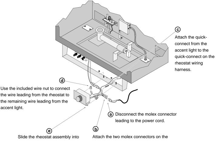
Slide the rheostat assembly into place and secure with the included nuts.
