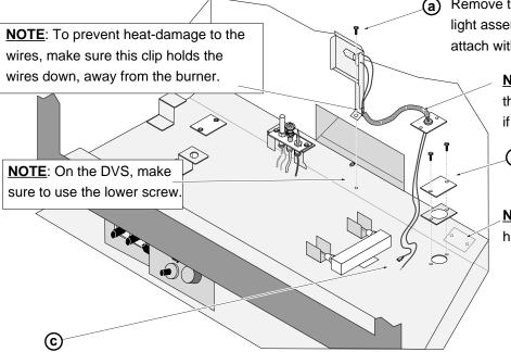
Remove this screw, position the accent light assembly in the same location, and attach with the same screw.
